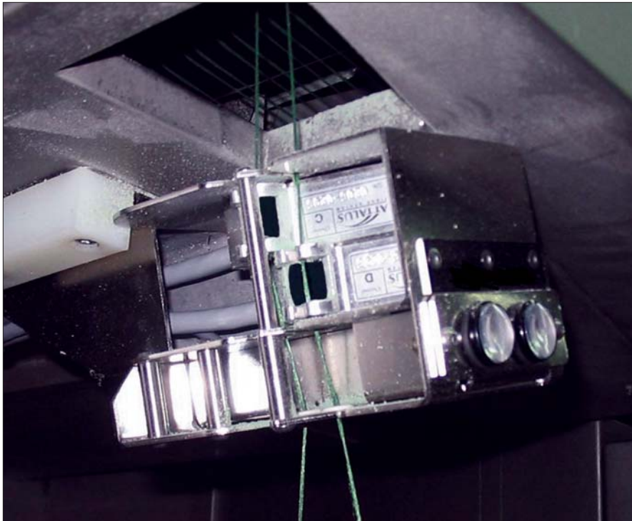
The Attalus system monitors and provides information on 100% of the carpet fiber produced.
